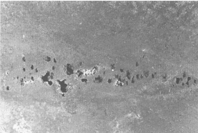
Figure 7.49 External cavitation corrosion on a cast iron cylinder lining in a diesel engine. 2 \times . (Photo: E. Abusland, Sintef Corrosion Centre.)
